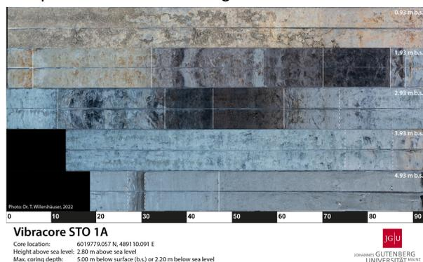
Figure 2: The Vibro-Core-Sample shows clayey silt, sometimes mixed/alternating with organic matter in the first 2.35 m, artificial deposition, H. Hadler [3]
