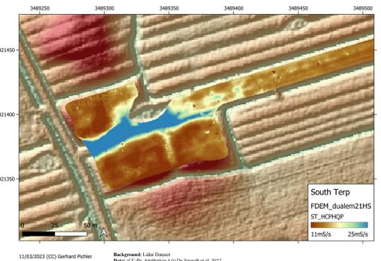
Figure 5: Higher conductivity zone splits the two south terps
