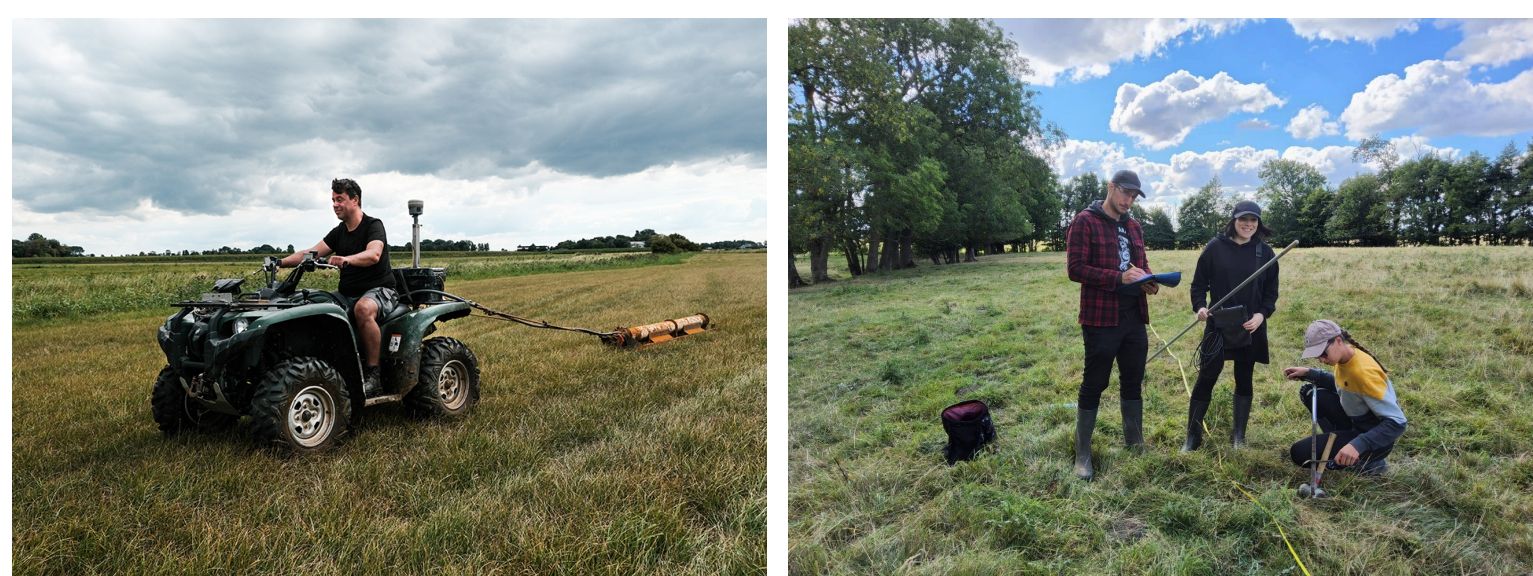
Figure 2: Electromagnetic interference (EMI) measurements and soil sampling near the Tofting terp.
